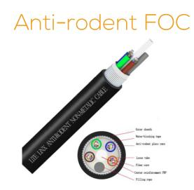
The cable's core features a non-metallic central core made of Fiber Reinforced Plastic (FRP), which provides structural stability. To maintain a compact and circular cable core, the loose tube and filler rope are precisely helically wound around this central reinforcing core, ensuring the cable's shape and integrity.
