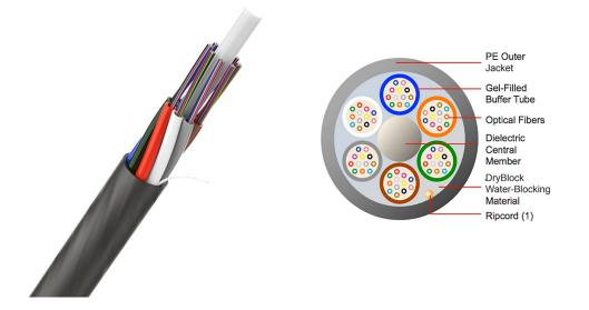
This ABF Cable product offers impressive mechanical and environmental characteristics. It boasts lightweight construction, a small diameter, and a high optical fiber capacity of up to 288F. Additionally, it features a low sheath friction coefficient. This cable is designed for installation into micro-ducts by using an air-blowing machine, making it ideal for micro tubes with a diameter of approximately 14/10mm.
